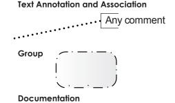
A **Text Annotation** is a comment visible in the diagram, linked to a diagram node via an Association connector.
